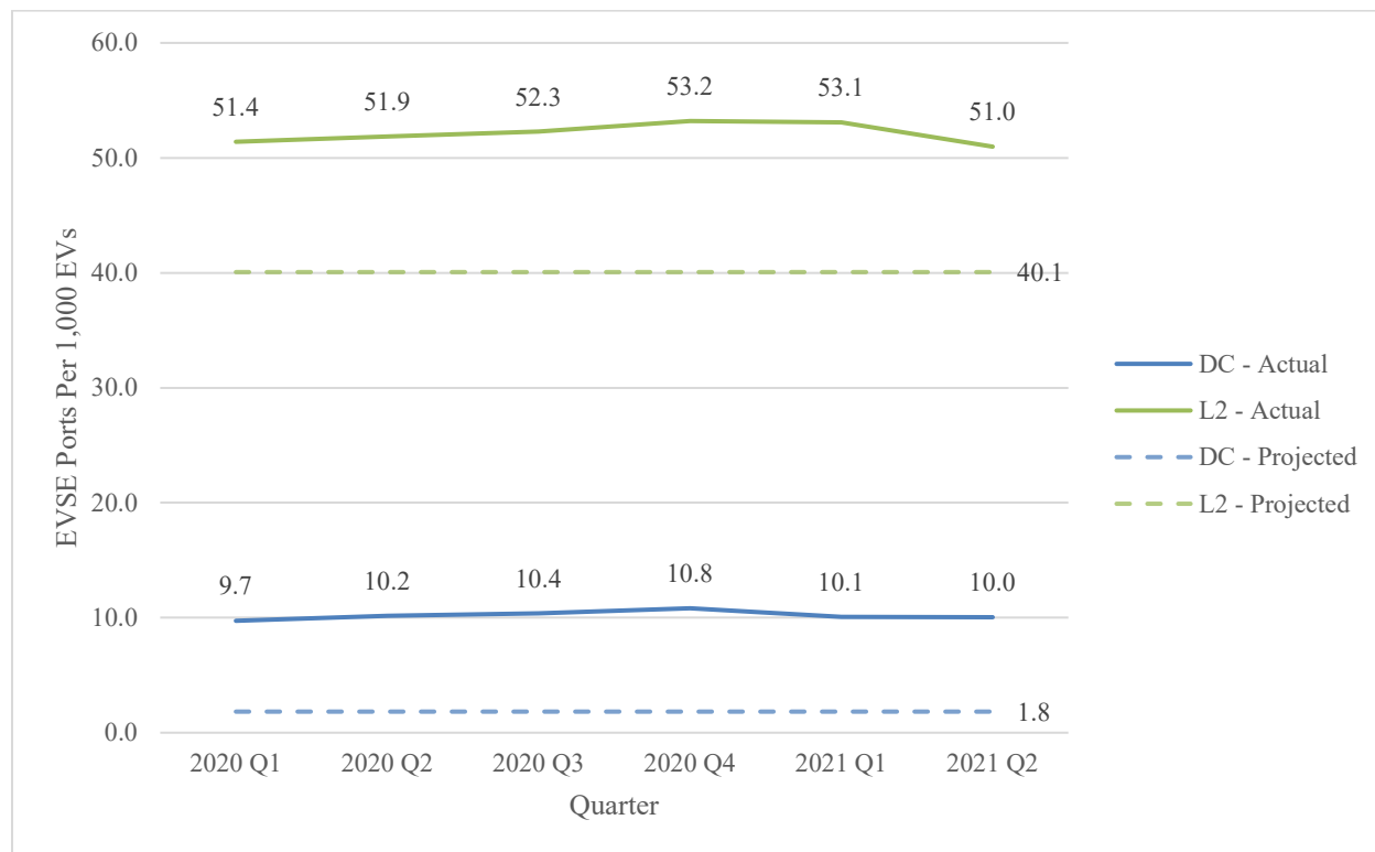
Figure 19. Quarterly availability and projected 2030 need of public and workplace EVSE ports per 1,000 EVs in the United States to support 15 million EVs 5
